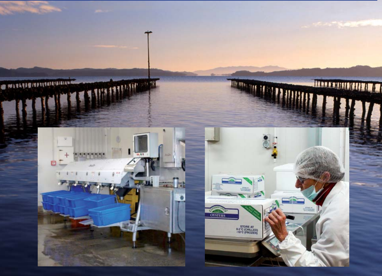
Oysters are graded before processing by a computer controlled sorter. Different sizes are processed separately.
